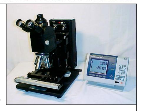
illumination simultaneously. This method of multi Bright and Dark Field illumination combinations enables detection of all defects in a single manual scan not found in common Bright Field mode inspection microscopes.
